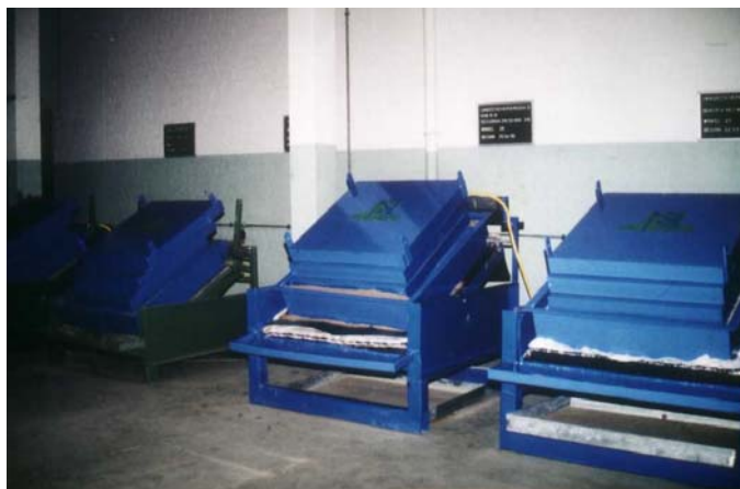
Fig. 4: Long-term shear boxes with Bentofix® type B
